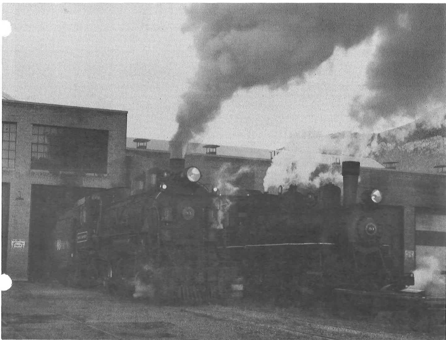
Nevada Northern No. 40, a high-driver 4-6-0 designed for passenger service, sits by the newly restored 2-8-0 No. 93, designed to pull heavy ore trains from the copper mine to the smelter. The two locomotives were steamed up and made ready for the railroad's first photographer's special on October 8, 1994. (Kenneth Jessen Photograph)
