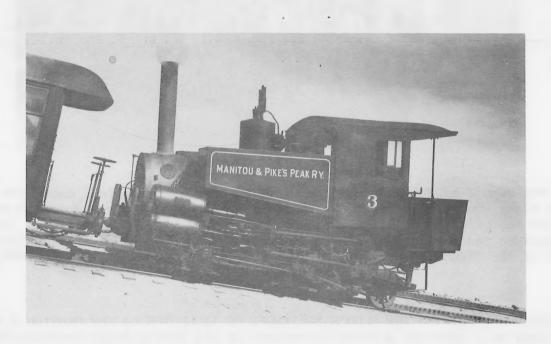
Manitou & Pikes Peak Railway Locomotive No. 3 at the top of Pikes Peak, on August 27, 1939. This 0-4-2 rack and adhesion engine had been rebuilt by Baldwin in 1893 as a four-cylinder Vauclain compound. (Dick Kindig)
