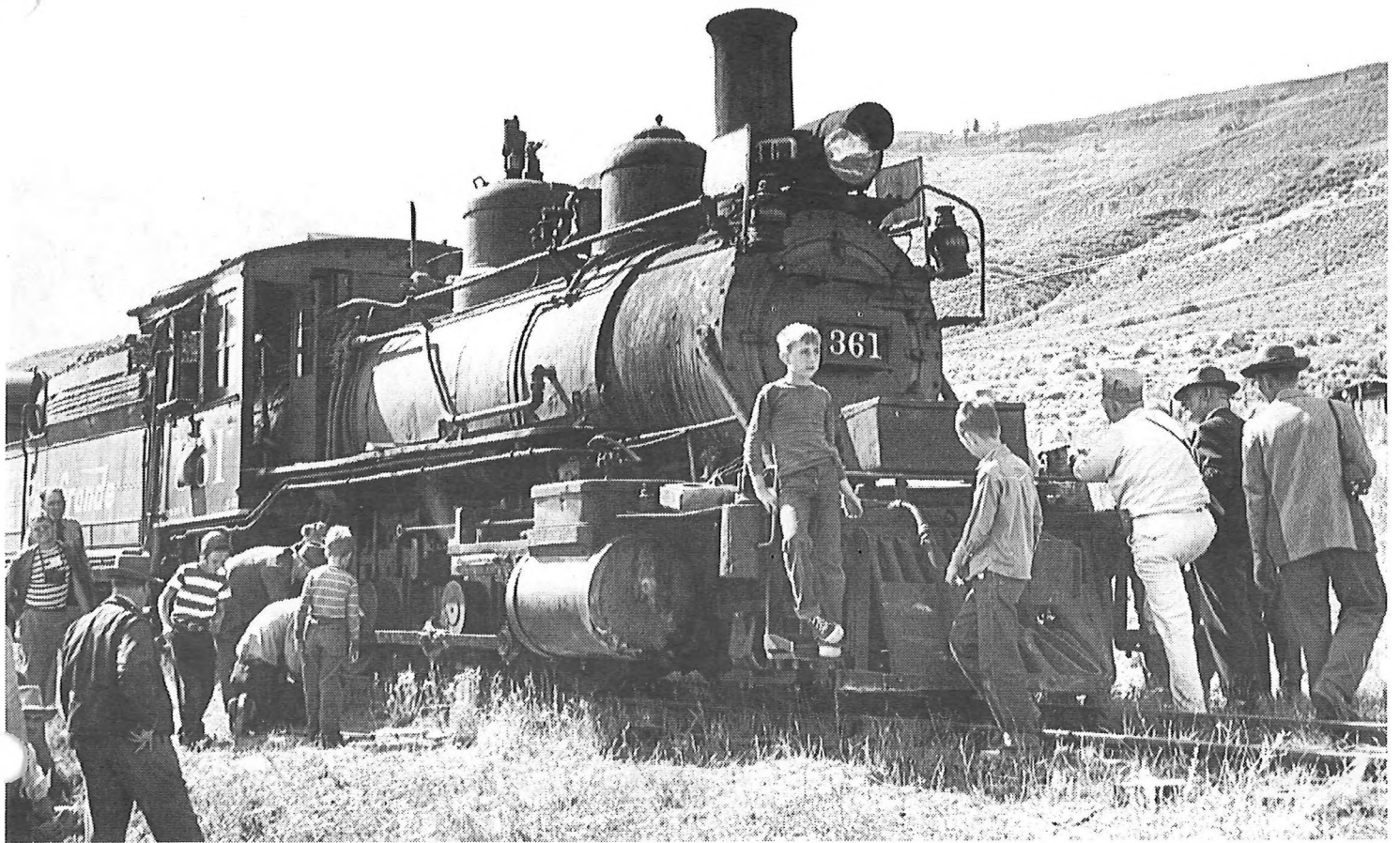
Trouble rears its ugly head on a Rocky Mountain Railroad Club trip over the weekend of September 18-19, 1948, on a round trip from Salida to Gunnison and Cimarron. On the return trip, the 361 suffered a broken slide valve. As the RMRRC members, friends and family await their rescue, the engineer and fellow railroad official take down the main rod to allow the engine to be towed. The younger rail fans are offering their advice, and/or supervising the work at hand. (9/19/48) (Cornelius W. Hauck Photograph)
