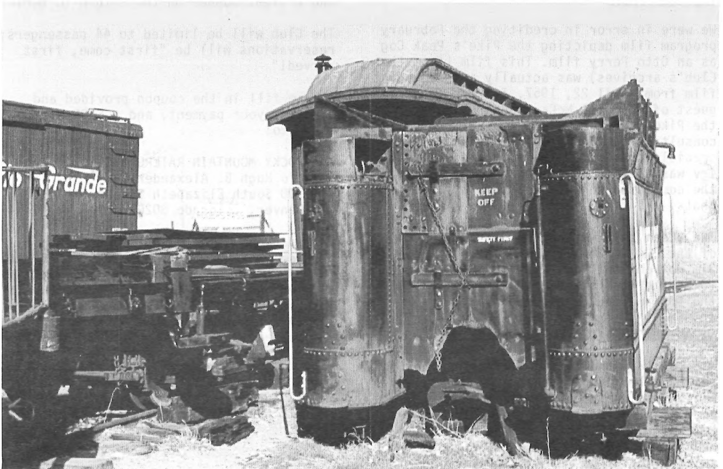
The Club's Rio Grande Southern #20's tender is one of the major projects scheduled for the annual Work Weekend on June 14 & 15, 1997, at the Colorado Railroad Museum. Decking has to be applied to the tender frame, and, the tank will have to be lifted back onto the deck.
