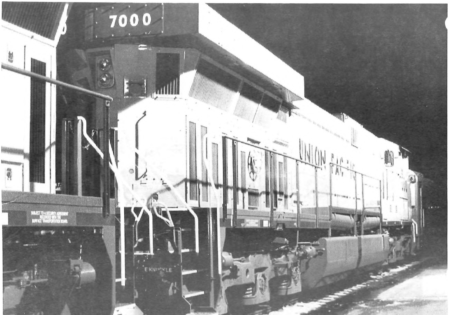
Union Pacific AC6000CW's 7000 and 7003 are shown in a night shot in the UP's (ex-SP/D&RGW) North Yard on November 17, 1996. The engines had been on ex-D&RGW lines in Colorado going through performance tests. (Chip Sherman Photograph)
