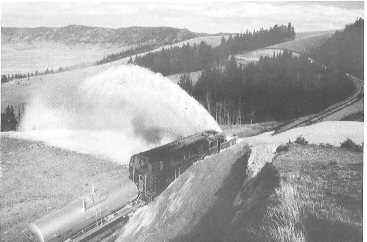
Union Pacific's Rotary Snowplow #900082 is seen at the Loops above Albany in this May 5, 1996 photograph. Along with two UP SD40-2's and a Conrail unit, the ex-UP Coalmont branch (currently the Wyoming Scenic Railroad, ex-Wyoming & Colorado [WYCO]) was cleared of remaining snow drifts (some as deep as eleven feet) so that final operations can be cleaned up prior to abandonment this fall. (Steve Rasmussen Photograph)
