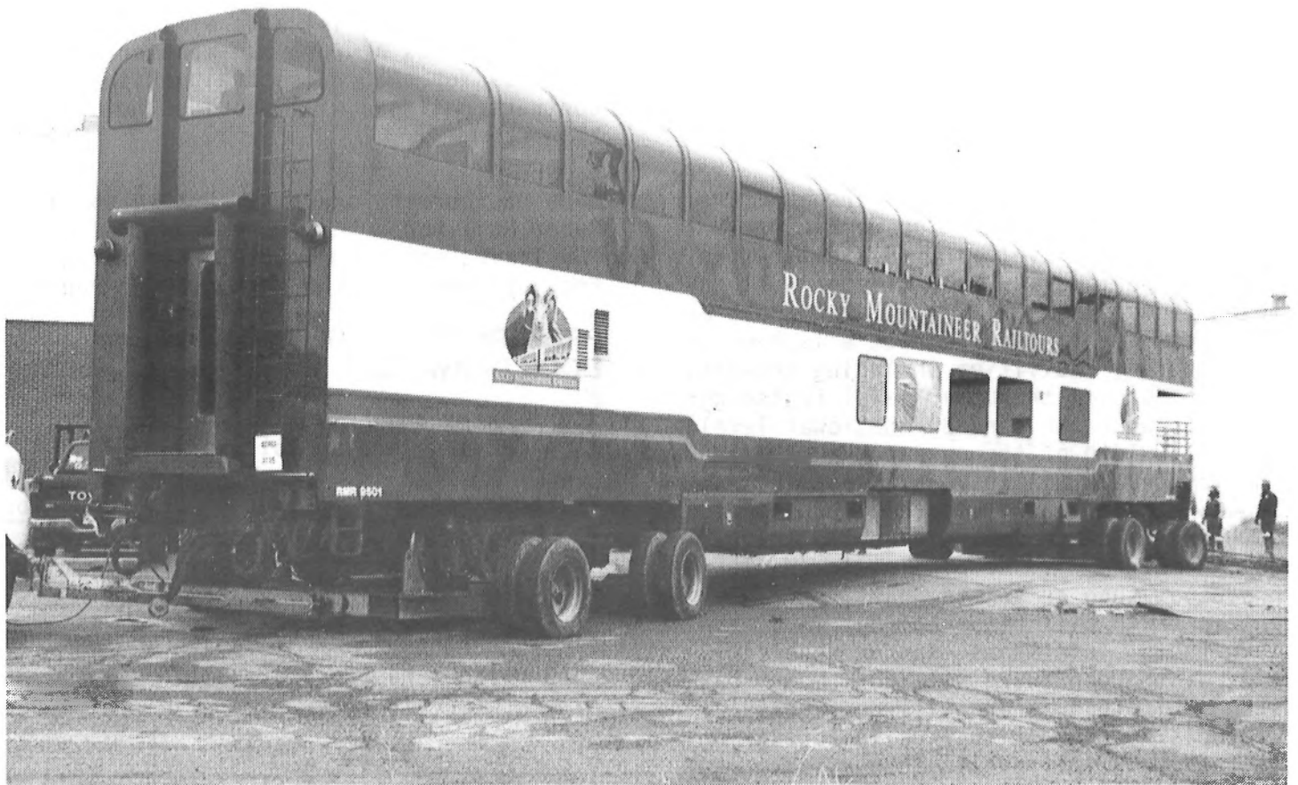
A definite highlight of the Rader Rail tour was the transfer of the Rocky Mountaineer rail car from the construction floor to the rail track service line via rubber tired trucks. We were quite impressed on how they maneuvered these 100-ton cars. (Alan Greene Photograph)
