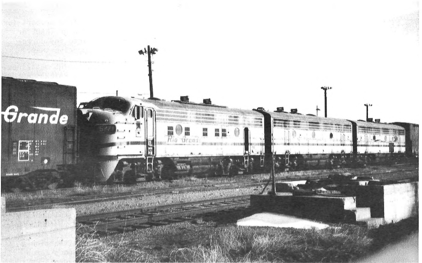
Taken in February, 1994, the above photo shows "Rio Grande" EMD diesel locomotives F9A 5771 and B-units F9B 5762 and 5763 sandwiched in between boxcars on the storage track on the west side of the Southern Pacific/Rio Grande Burnham shops. By 1973, the only remaining "F" units on the roster, they were the motive power for the RIO GRANDE ZEPHYR which saw service until 1983. Memories bring back the enjoyment we all experienced and the sadness too, to see them in service for the final time on the Zephyr during the Club's April 23 & 24, 1983, excursion to Glenwood Springs, Colorado. Sitting idle all these years, we wonder what their final disposition will be. (Joe Priselac) [Your editor votes for the Colorado Railroad Museum--how about you?] (Joe Priselac Photograph)
