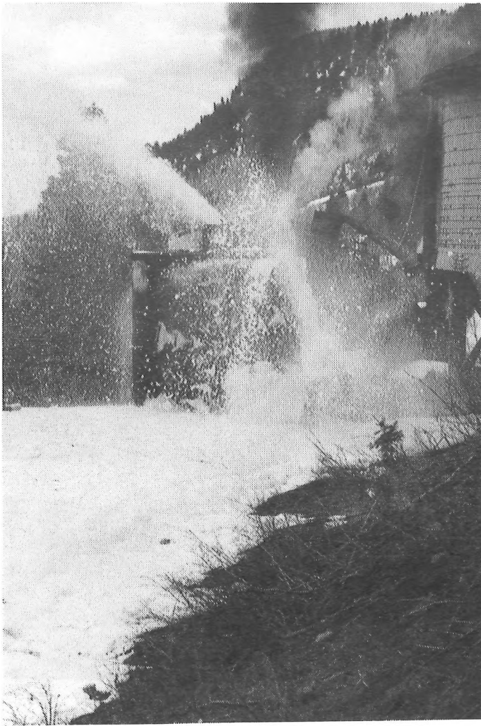
The Rotary Train has reached Cresco Water Tank. The Rotary was pushed just enough to get it and each of the three engines up to the water tank before serious plowing was resumed. It was a wonderful experience to witness all the operation of watering the four tanks with Rotary action in between each stop for water. (Jim Trowbridge Photo)
