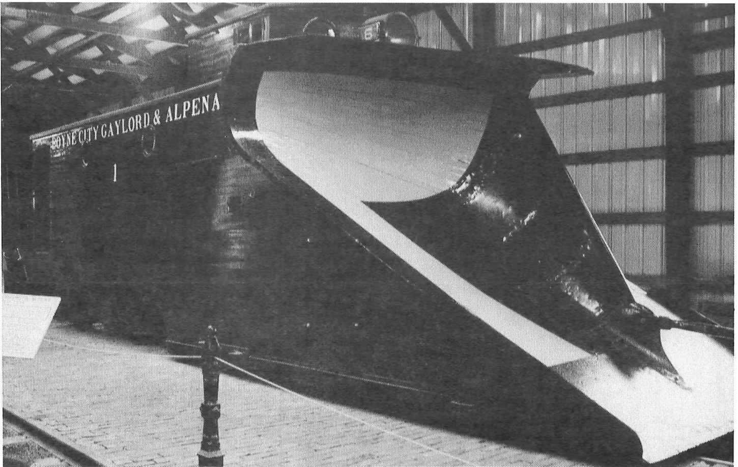
This Russell snowplow was built in 1906 by the Russell Car & Snow-Plow Company, Ridgeway, Pennsylvania. This early snowplow is of all-wood construction with the exception of iron plates covering the actual plow surface. Before being acquired by Mid-Continent in 1977, this RUSSELL plow spent its entire life working the upper part of lower Michigan on the Boyne City, Garlord & Alpena Railroad (later known as the Boyne City Railroad when the line abandoned its trackage to Alpena in 1925). It was their Snowplow No. 1. The plow was last used by the railroad in the winter of 1958. (Sherm Connors Photograph)
