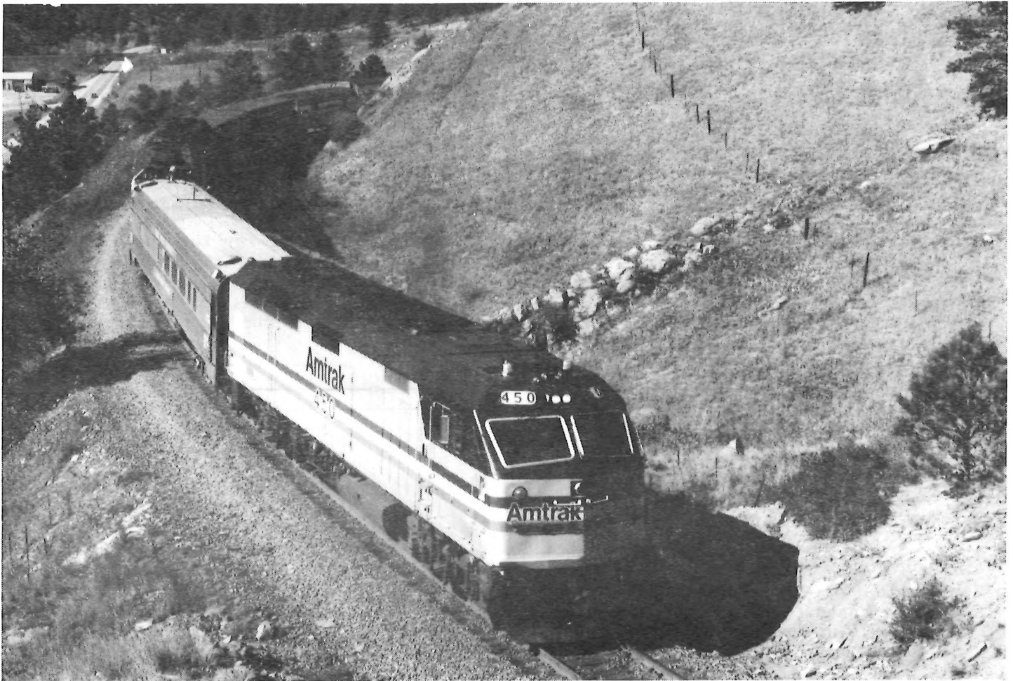
Amtrak #450 F-69PH, with AC Traction Motors, entering Tunnel No. 1 on the D&RGW's Moffat Line on October 10, 1990. General Motors "Electro Motive Division" test car ET840 is between F-69PH numbers 450 and 451 on the Westbound California Zephyr. (Joe Priselac Photo)
