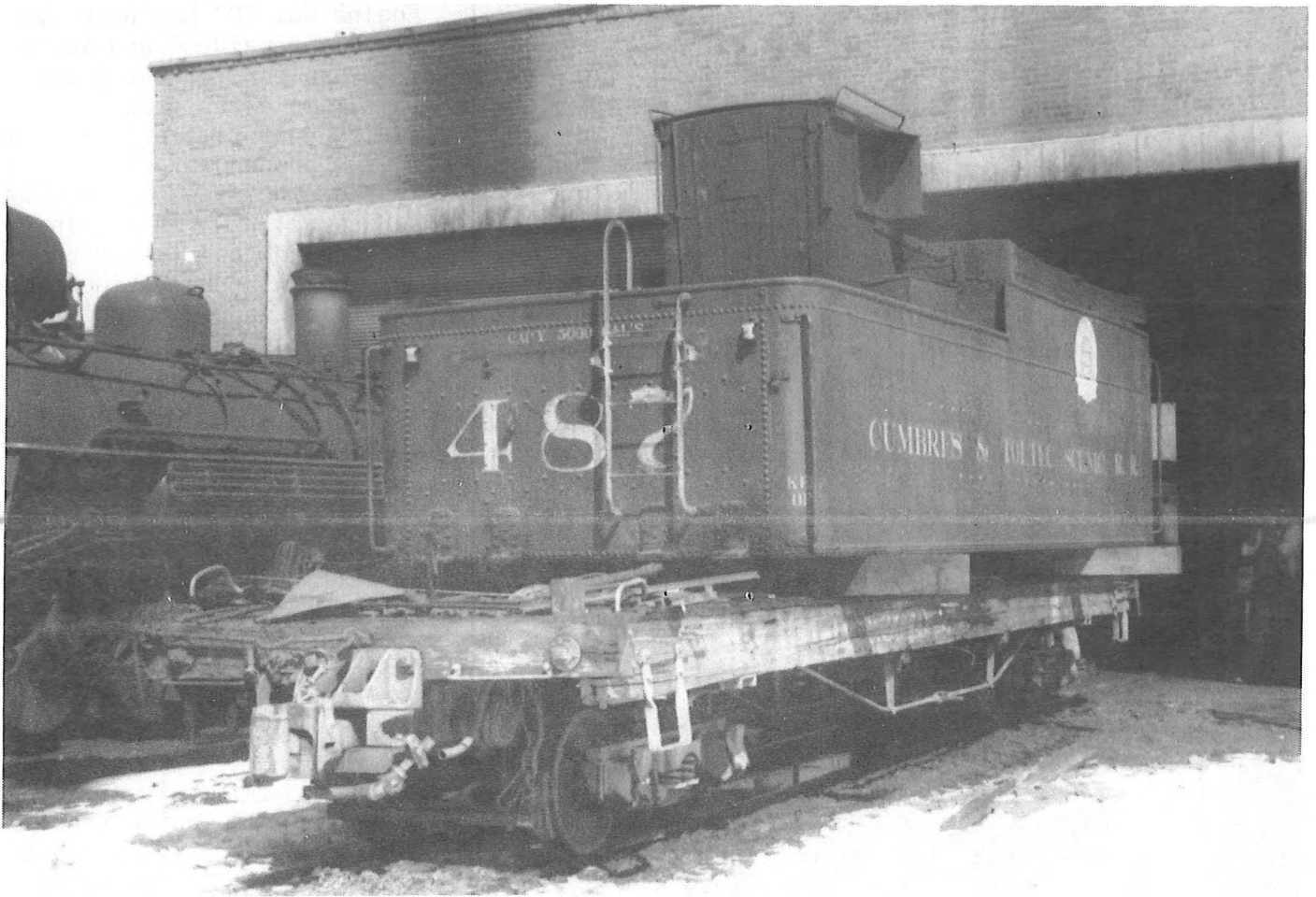
The tender wrapper has been fully removed from tender No. 487 and will be stored in the yards until disposition is determined. The wrapper may find eventual use in MOW service. (Earl Knoob Photograph)
