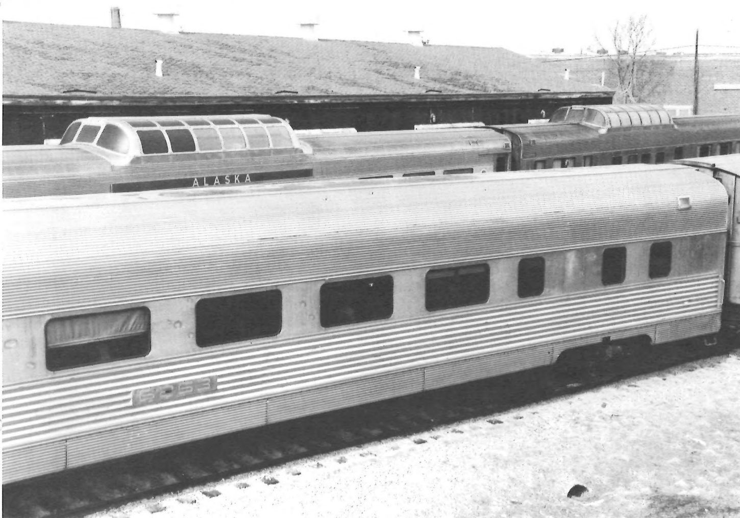
The largest collection of Budd stainless steel in the U.S. today has been collected by the Roaring Fork Railroad Company in preparation for the proposed route between Denver's Stapleton International Airport and Aspen, Colorado. Amtrak #5627, foreground, (Budd-built 1946, 56-passenger coach, built as FEC Jacksonville ) and ex-Alaska Railroad dome, 46-seat coaches #'s 7032 and 7022, are part of the growing fleet. Photo taken on March 4, 1987 at the Rocky Mountain Arsenal by Chip Sherman.
