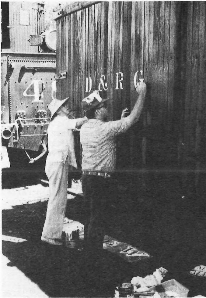
Box Car No. 3585 receives a new lettering job from (l to r) Barbara Whitmore (RMRR Club) and Jim Trowbridge (RMRR Club). The stencils could not be sprayed without running, so the lettering was traced and filled in by hand-painting. What a job!
