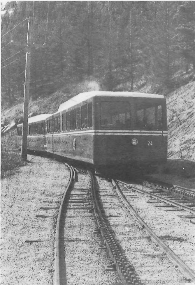
Our second photo run-by, showing the unique track with cog rail. This was done at the Minnehaha switch.
