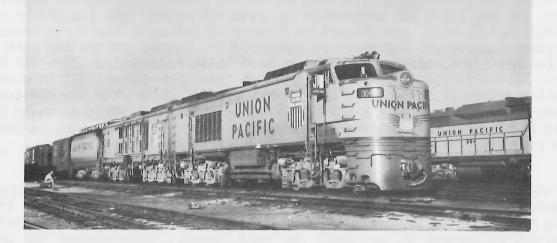
Do you remember these big beauties? Dick Kindig photographed the Union Pacific's gas-turbine electric #1 at Cheyenne, on October 13, 1962. Delivered to the UP in 1958, these 8,500 hp "Big Blows" were two units, permanently coupled and equipped with auxilliary heavy oil tender.
