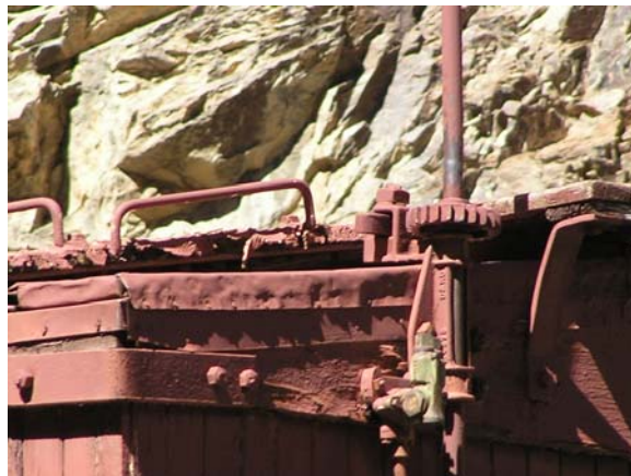
Figure 89. Re-welded hand brake needs to be ground flush and repainted
