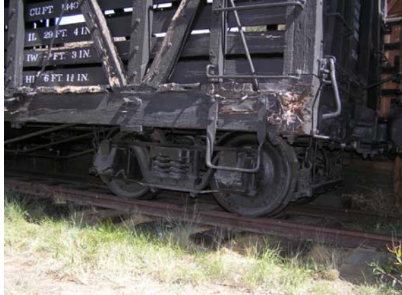
Figure 112. Undercarriage and rotten A end beam
