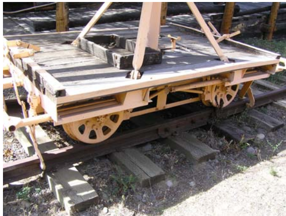
Figure 128. Undercarriage of crane car
