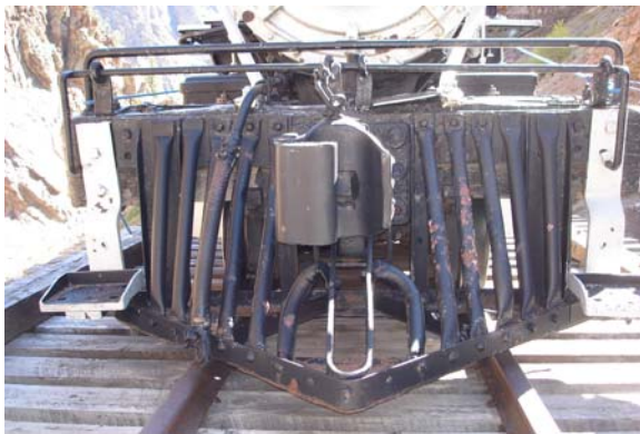
Figure 69. Paint peeling and rust on pilot and bars
