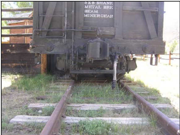
Figure 106. B end cupola, end beam
